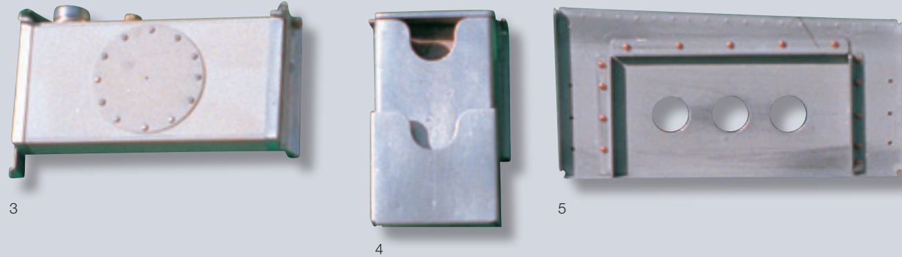
Some of the many minor cockpit components completed and awaiting painting: I made the de-icing fluid tank (3) from polystyrene, but the map case (4) and accumulator tray (5) are folded from litho plate.
