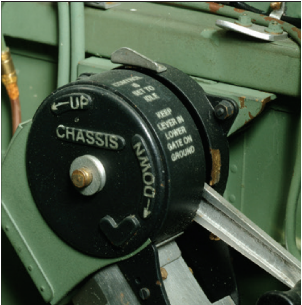
The undercarriage selector gear provides an excellent example of the use of dry transfers. However, great care and patience are needed to apply the tiny rubdowns to awkward surfaces. Wastage must be anticipated, which is why it is better to make more than needed.
