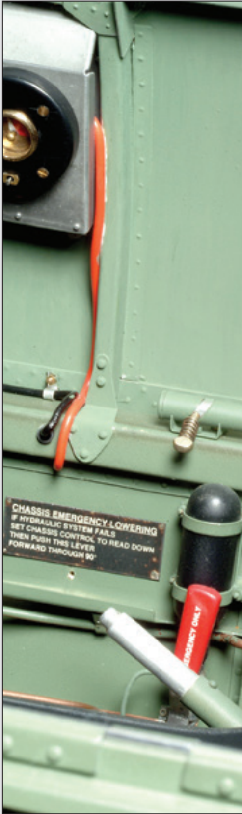
These pictures of the port and starboard cockpit walls nicely differentiate the use of dry transfers and photo-reverse reprographics to create labels as detailed in the text. Note how the placards have been weathered, and the addition of tiny fasteners attaching them to the airframe, just as in full size practice.
